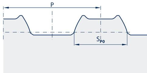
Tools with **splineshaft profile** gear-cutting with bump and chamfer
