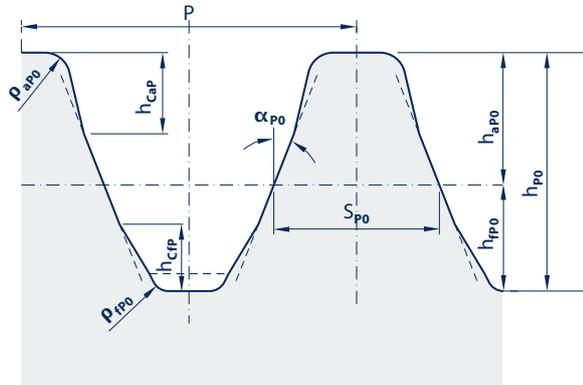
Tools with **tip and root relief** for more silent running and for avoiding contact impact.
