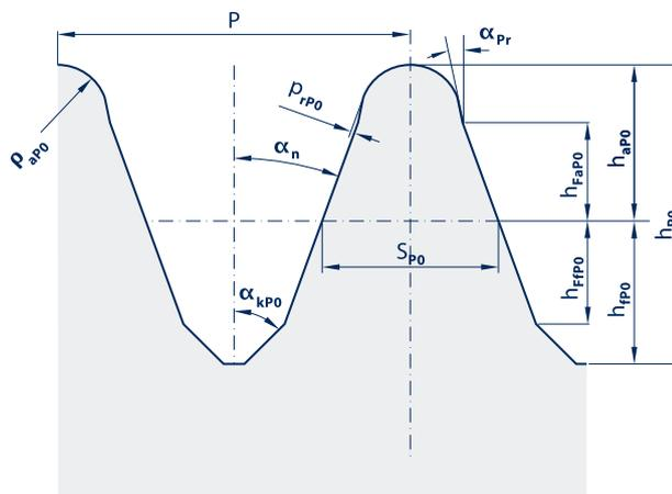
**Protuberance tools** for involute gears with tip chamfer and flank allowance with simultaneous root cut for subsequent finishing, e.g. honing or tooth flank grinding.
