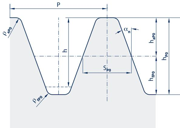
Tools with **standard profile** for involute gears. For making spur or helical gears with or without finishing of the outside diameter of the workpiece (see also Stock List)
